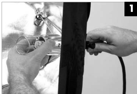
With Rifa on stand, and unplugged, grasp rear stem firmly with one hand, and lamphead with the other.
